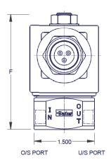
3/8-24 UNF 2B, 9/16" hex (2-Way Normally Closed) or 3/8-24 UNF 2B, 11/16" adapter (other configurations)
